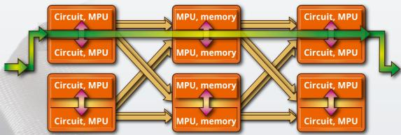
The green arrow shows signal path when a failure occurs.
